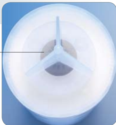
RFID tag embedded in a Millipore SMART filter
