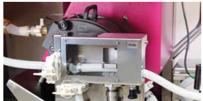
Figure 6. The Automated Pressure Control Valve (PCV) features a clear outer door enabling a clear view during operation. If the door is opened during operation, the valve automatically shuts off ensuring operator safety.
