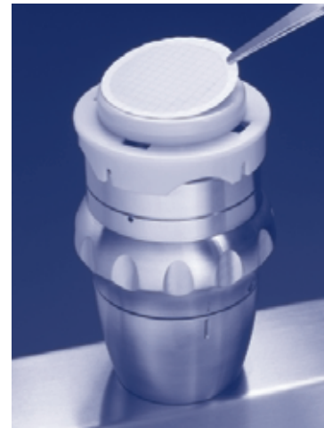
3. Incubate the membrane by lifting the membrane and transferring it onto a media plate.
