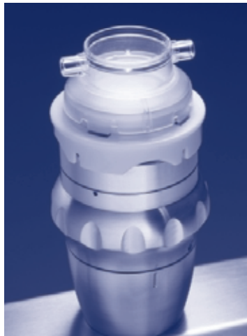
2. Access the membrane by connecting the MSOpener™ to a vacuum source, and placing the MicropreSure In-Line Filtration Sampler on top of the MSOpener.
