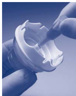
3. Insert broth medium via the base or the dome and remove any excess media with a syringe then incubate the MicropreSure monitor.
