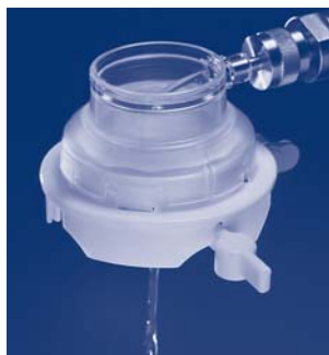
1. Sample directly through the MicropreSure monitor via the sanitary sampling valve.
