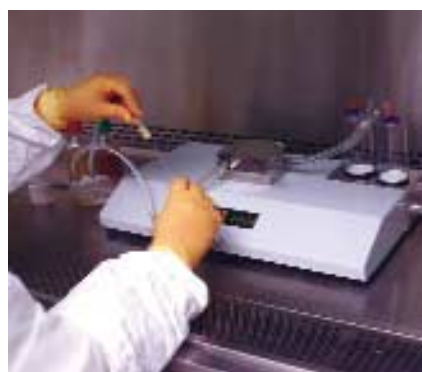
Connecting the NovAseptic bag with the Steritest instrument. MILLIPORE CORPORATION (WWW.MILLIPORE.COM)
