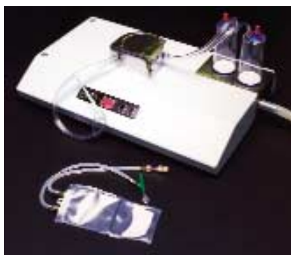
NovAseptic sample device and Millipore Steritest. MILLIPORE CORPORATION (WWW.MILLIPORE.COM)
