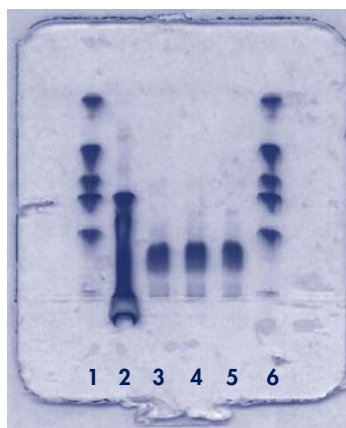
Figure 5. SDS-PAGE gel of a purified IgG (overloaded) to show any variations over 100 cycles.
